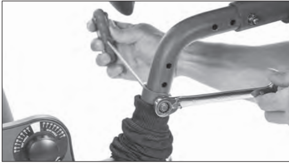
9. Using hex wrench and 13mm wrench tighten securely.
